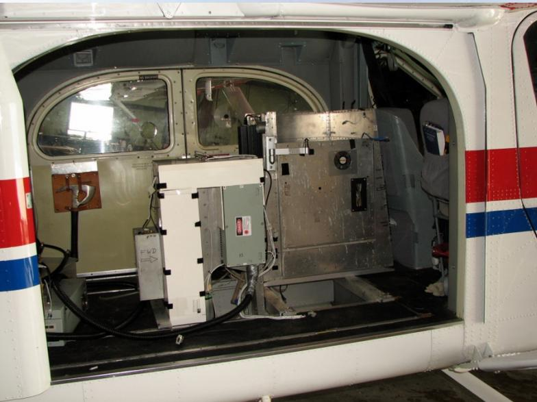
USGS Topographic/Bathymetric Lidar (EAARL)
