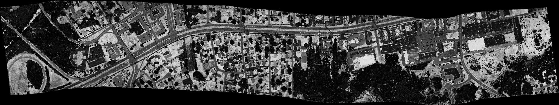
Point cloud color-coded by intensity in QT Modeler
