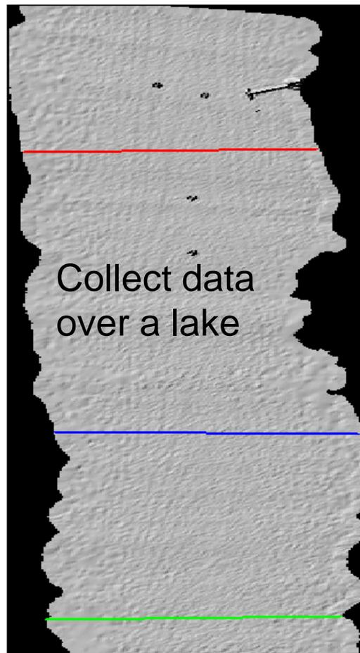
A frown in a profile from the water points indicates scanner mirror angles are being under-reported
