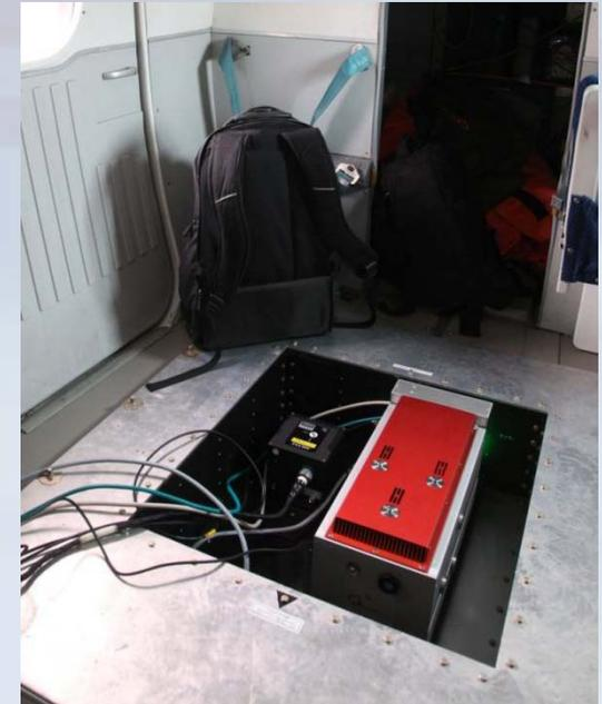
Riegl Topographic Lidar (LMS-Q680)
