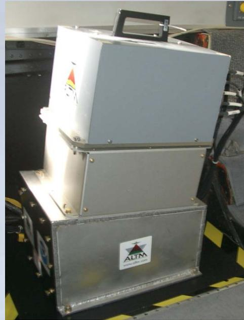
Optech Topographic Lidar (ALTM 2050)
