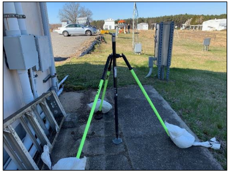
Fixed-height range pole
