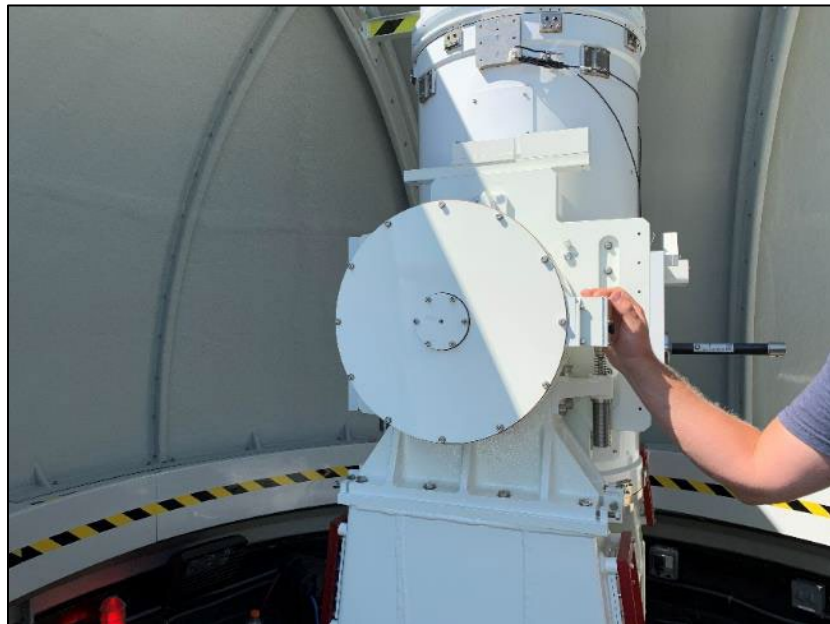
Elevation Reference Point
