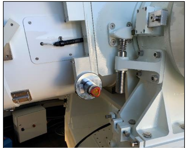
SGSLR with mounted reflector. Targets were positioned as they scribed circles about the azimuth and elevation axes
