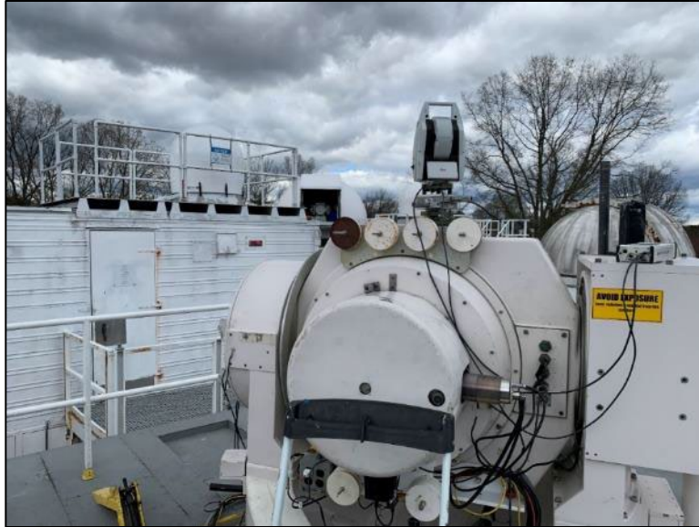
AT402 Laser Tracker mounted on MOBLAS-7
